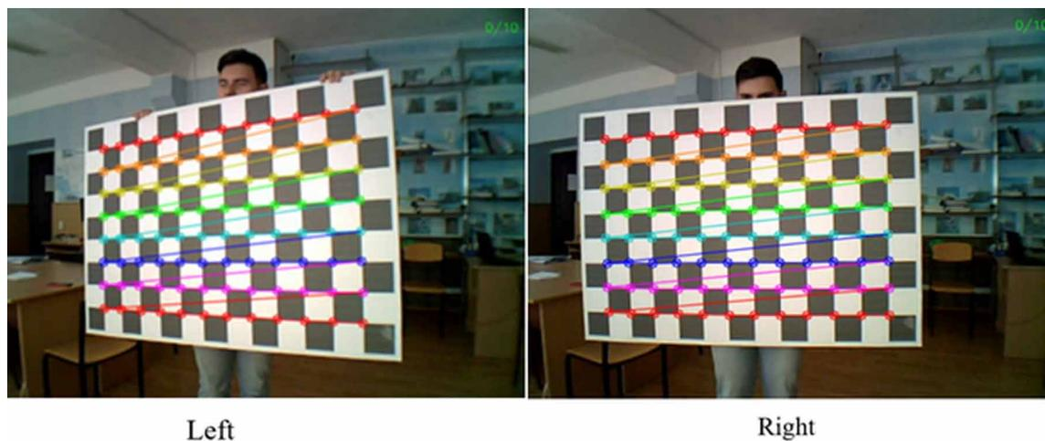
After that, for images on which the corners of the chessboard were successfully found, it is possible to calibrate each camera separately using the following procedure:
